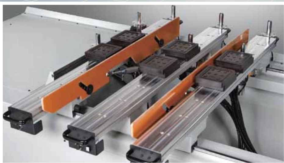
A laser positioning system is used for automatically positioning beams and suction cups. Panel lifting blades make easy work of positioning and moving heavy work pieces.
