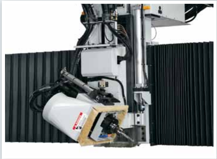
Anderson's NC series allows for any size machine to be engineered and constructed. Multiple axis machine designs are product specific and completely adaptable to a customer's needs in a machining center.
