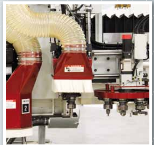
Various line boring unit, spindle and tool carousel combinations allow customers to configure the machine for their specific application and budget.
